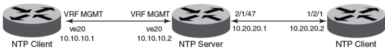
FIGURE 4 Use case 2: NTP server over Management VRF with one client using Management VRF and another client using Ethernet
